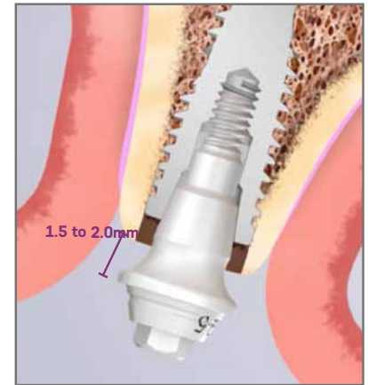
Figure 12. Abutment margin with a safe distance from the bone crest (minimum 1.5mm).
